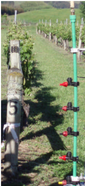
Five nozzle boom used for mealybug application.
