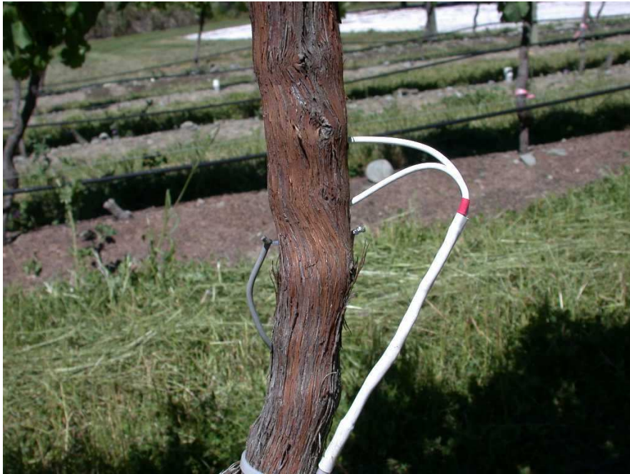
Figure 1. A total of 18 sets of sap flow probes were installed into the vines at the trial site at Nautilus Estate. Sap flow was measured once every 30 minutes using the T-max heat-pulse method (Green et al., 2003).
