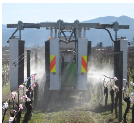
Figure 13. Applying pruning wound protectant with a sprayer.
