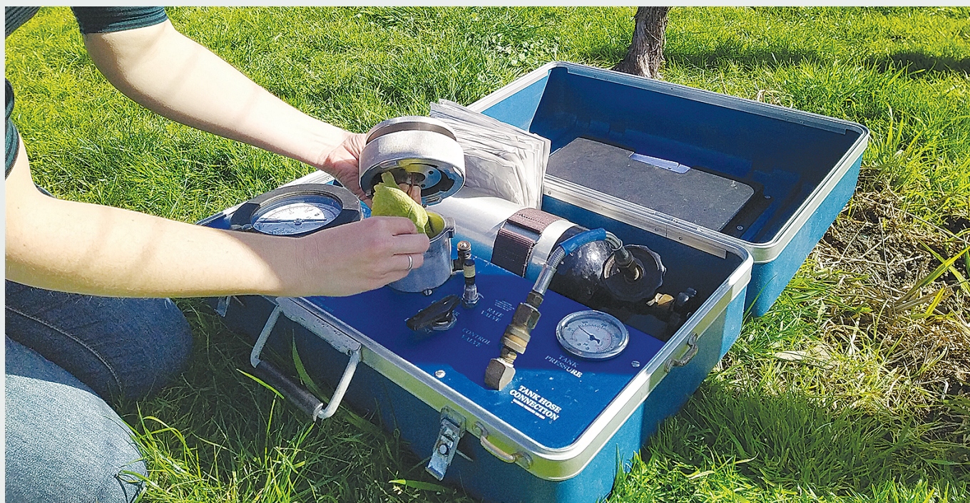
Figure 1. Pressure bomb measurements were done in the vineyard to assess irrigation timing
