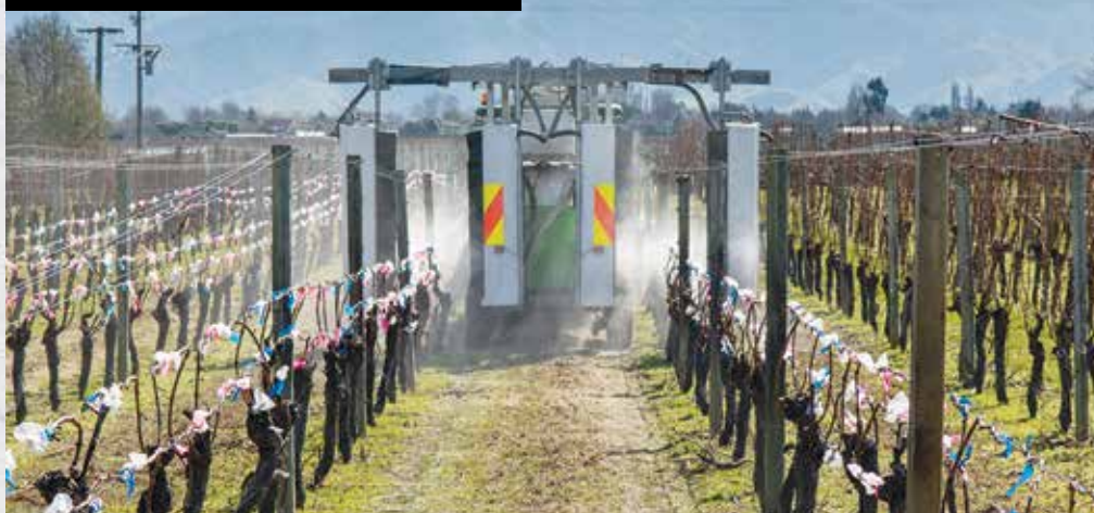
Figure 6. Recycle sprayer applying fungicides to pruning wounds in the Marlborough vineyard trial.
