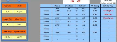
**0.5m** loss through 2m of 25mm pipe
