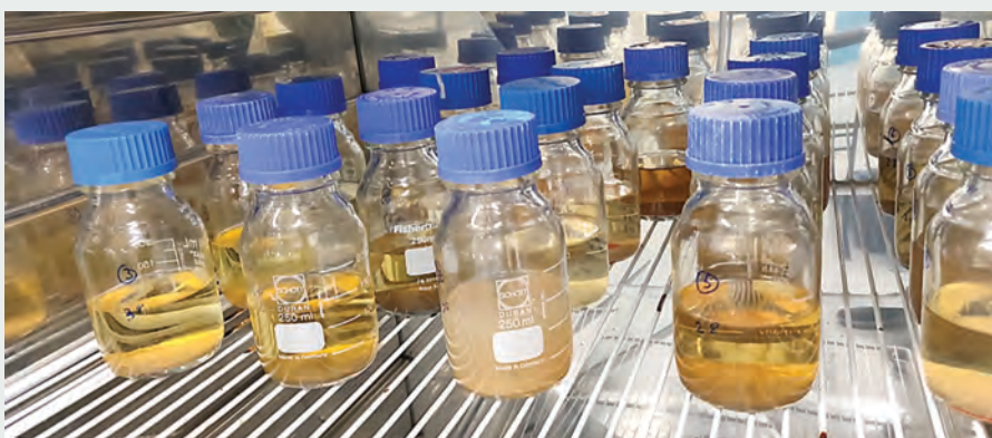
In this experiment, the additions of flavanols (catechin and epicatechin) and tannins were used to establish and test the lab-scale maceration and fermentation system
