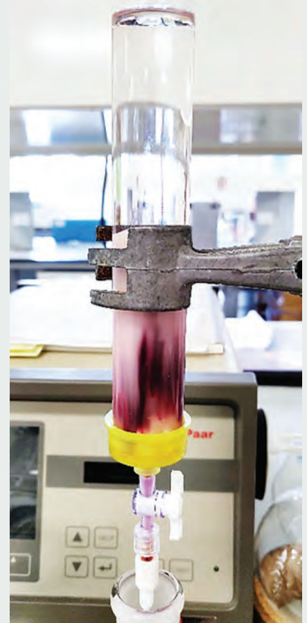
Extraction of monomeric anthocyanins from Pinot noir grape skins using solid phase extraction.
